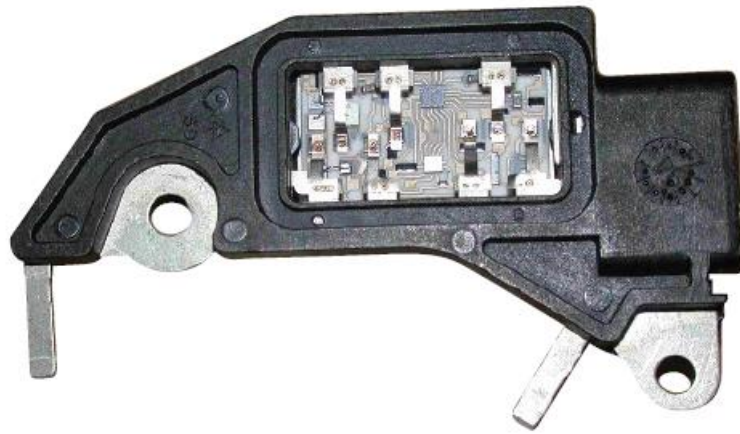
Figure : A typical electronic voltage regulator with the cover removed showing the circuits inside.
